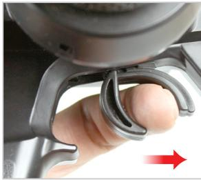
Extend the trigger on the Tx forwards. The wheels should rotate in the direction to drive the model backwards. If prior to doing this, the model was traveling forward, the model's breaks will activate rather than shifting the model directly into reverse.
