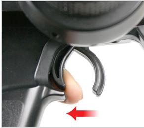
Slowly and evenly squeeze the trigger on the Tx and the wheels on the model should drive the model forward.
