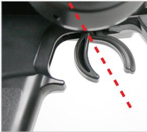
Release the trigger on the Tx and the motor should idle and the car should gradually roll to a stop.
