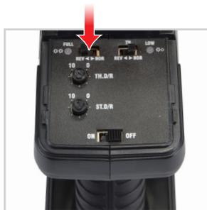
If needed, to reverse the steering servo control direction, move the steering reverse switch to the opposite position.
