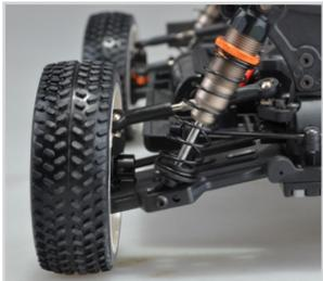
Various shock springs are widely available in the market. Springs provide various elasticity and modify the performance of the suspension system.
