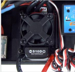
The stock electronic speed controller is specially matched with this model and requires no setup, programming, or special calibration.
