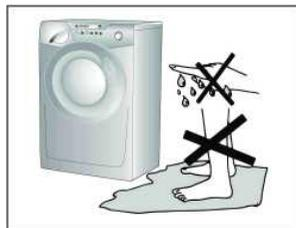
m. Check there is no water left in the drum before opening the door;
