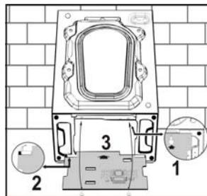
**N.B!** If the appliance is installed on a carpeted floor ensure that the ventilation holes on the sheet are not obstructed.
