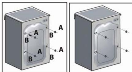
**Note:** we recommend you keep the spacers and screws to immobilize the machine for future transit. The Manufacturers will not be responsible for any possible damage to the machine caused by not following the rules relating to releasing the mechanism. The user is responsible for all costs of installation.
