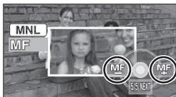
The centre of the screen is enlarged. The normal screen returns approximately 2 seconds after you finish bringing the subject into focus.
