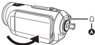
The status indicator **A** goes off and the power turns off. (If [QUICK START] is set to [ON], the unit goes into quick start standby mode and the status indicator lights green.)
