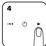
If jam occurs, press and hold forward (▶) button until the document is completely through the shredder
