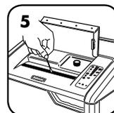
5 Using cotton swab, wipe away any contamination from the paper sensors
