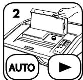
2 Press the auto and forward buttons at the same time for 3 seconds to manually oil shredder
