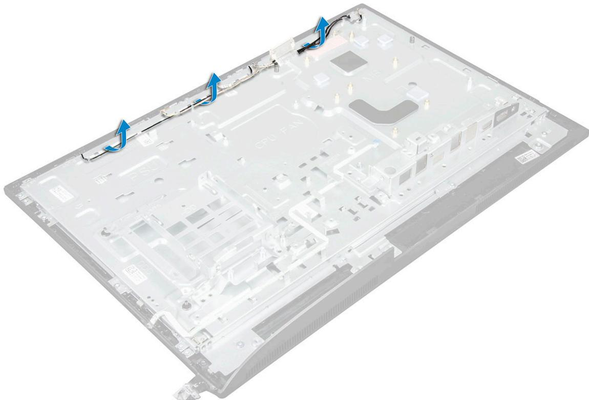
4 To remove the chassis frame:
