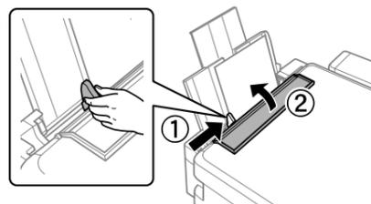
Slide the edge guide against the paper, and flip the guard back.
