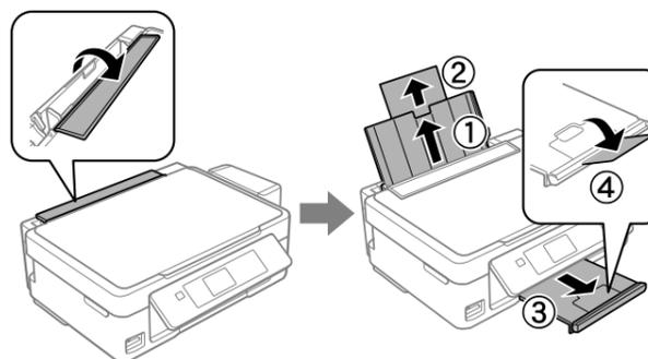
Flip the feeder guard, and then slide out the paper support and the output tray.
