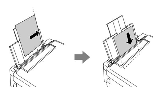
Load paper with the printable side face-up against the right side of the sheet feeder.
