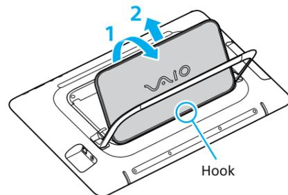
! After installing the battery pack, anchor the back panel to the hook, then close the back panel.
