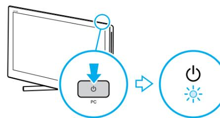
Press and hold down the PC power button until the PC power indicator light turns on.
