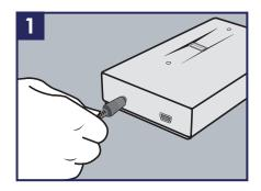
Connect the Hi-Speed USB Power-Sharing cable to draw extra power when necessary.
