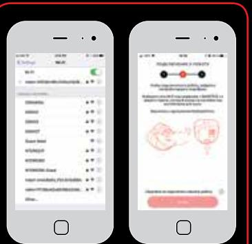
**EN** **To pair** the robot, go to your smartphone SETTINGS > WIFI Select SMARTFCEXXXXXXX Enter the Smart Force 8 characters password located under the dust container.
