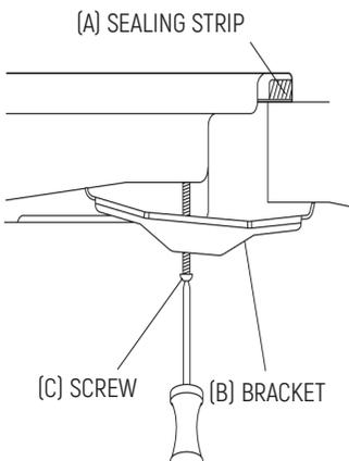
1. Place the bracket (B) over the holes that match the size of the screws. There are one set of screw holes in each corner of the hob (H). Slightly tighten a screw (C) through the bracket (B) so that the bracket is attached to the hob, but so that you can still adjust the position.
