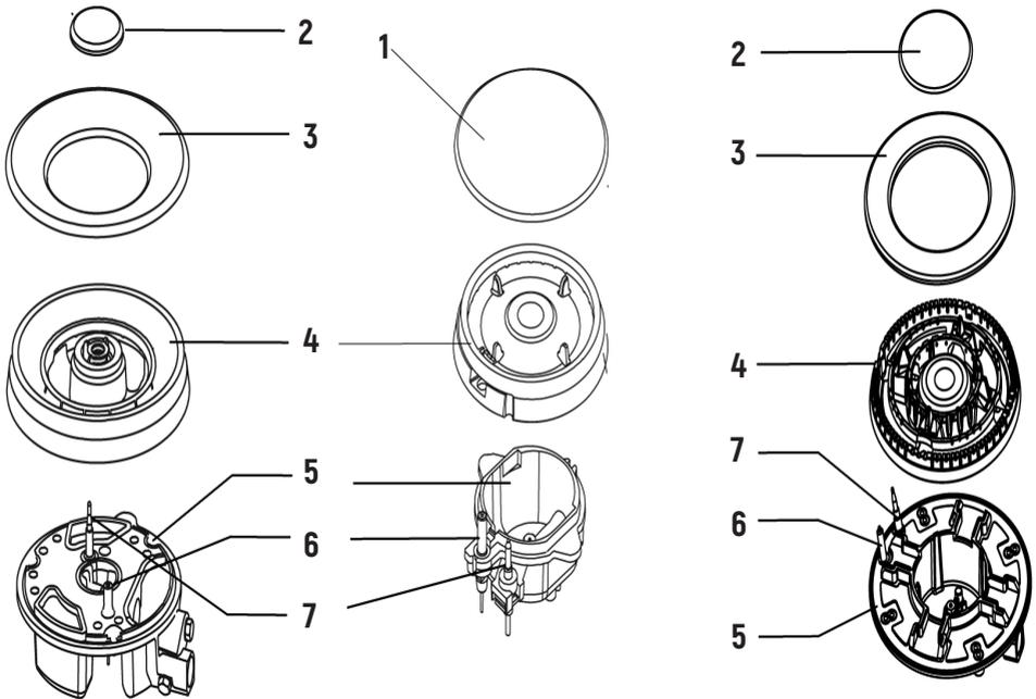
1. Place the flame spreader [4] on to the burner cup [5] so that the ignition device and the flame supervision device extend through their respective holes in the flame spreader. The flame spreader must click into place correctly.
