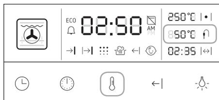
When you connect the meat probe, in each **function selector knob** position except CLEANING and **0**, the displays shows and the set temperature (80°C by default).
