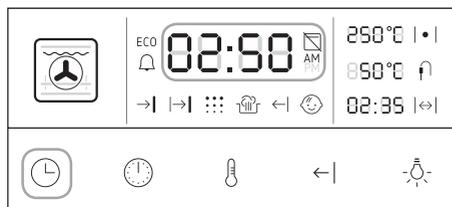
When you plug in the appliance there is a [confirmation] beep. Set the current time. The current time must be set for the appliance to operate. Touch controls or knobs do not respond. An [error] beep is emitted. You can only set the current time ⌚.
