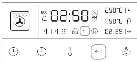
Use fast oven cavity heat-up to quickly reach the desired temperature. This feature is available in all **function selector knob** settings except DEFROST, CLEANING and «0». When you touch ←| in these settings, you will hear an [error] beep. When you touch ←| the heaters will be turned on and the appliance operates at the maximum power to quickly achieve the set temperature. FAST HEAT-UP symbol ←| is shown on the screen.
