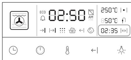
Additional timer display located in the bottom right corner of the display has functions, depending on the oven operating mode (when DURATION and DELAY START functions are active).
