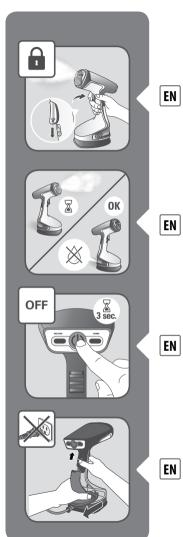
Put the steam trigger in the locked position.
