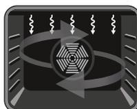
**Grill and Fan Function:** The oven's thermostat and warning lights will switch on, and the grill heating element and fan will start operating. This function is ideal
