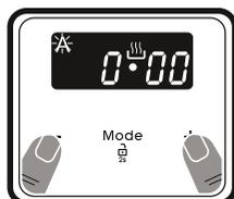
1. Press the "+" and "-" keys simultaneously. ☹ Symbol will appear, and the dot in the middle of the screen will start to flash.
