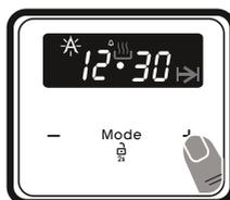
3. Use the "+" and "-" buttons to set the desired finishing time.
