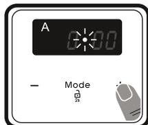
2. Adjust the time while the dot is flashing using the "+" and "-" keys.
