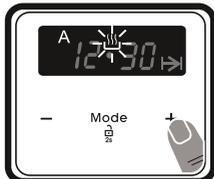
6. Select the desired finishing time using the "+" and "-" keys.
