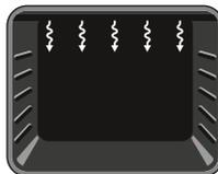
**Grilling Function:** The oven's thermostat and warning lights will switch on, and the grill heating element will start operating. This function is used for
