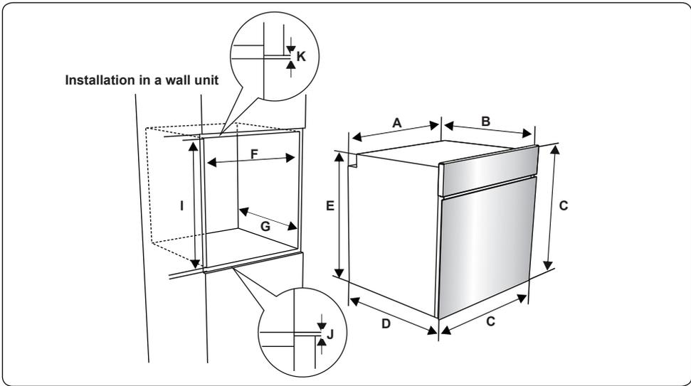
After making the electrical connections, insert the oven into the cabinet by pushing it forward. Open the oven door and insert 2 screws in the holes located on the oven frame. While the product frame touches the wooden surface of the cabinet, tighten the screws.
