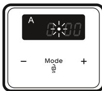
3. After a few seconds, the dot will stop flashing and will remain illuminated.
