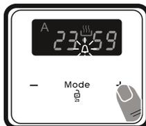
2. Select the desired time period using the "+" and "-" keys while 🔔 is flashing.
