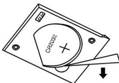
Attention: Do not bend the contacts – this can lead to their failure.
