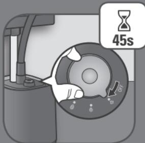
**EN** Turn the On/Off Button, in order to switch on the appliance. Then, adjust steam output by turning the button.
