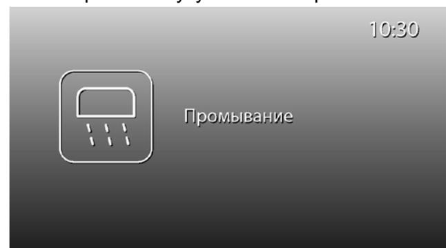
The **Rinsing** starts automatically after the switching of the appliance and also after other coffee machine functions.
