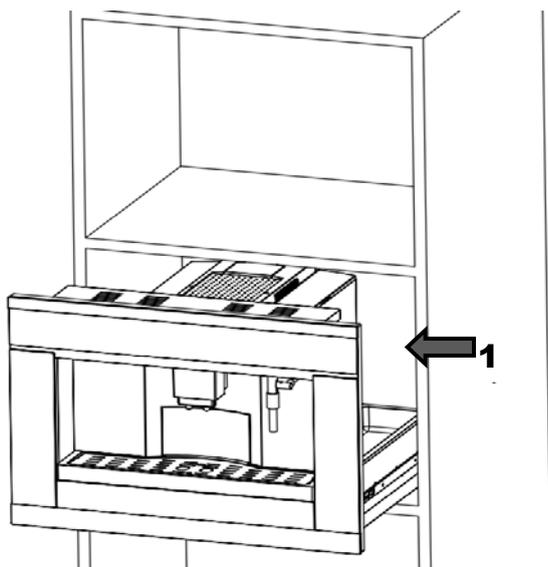
The water tank is located behind the control panel of the appliance on the left. To remove the water tank:
