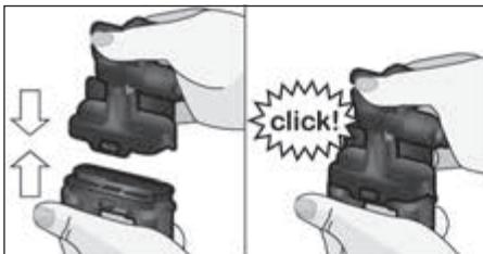
■ Place the milk system **4b** back in the appliance from the front, making sure it is straight.
