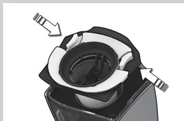
**4a. Cleaning of dust container and filters.** (Recommended every 5th cleaning). Release dust container, take out both filters by pressing release buttons.
