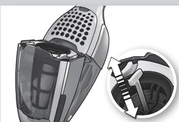
**3. Quick cleaning of the fine filter.** (Recommended every cleaning). Release the dust container, pull/release spring 5-6 times to dislodge dust.
