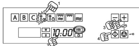
1. Press the function touch sensor Defrosting by time. The function key lights up.
