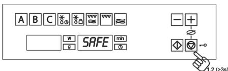
The oven functioning can be blocked (for example, to stop it being used by children).
