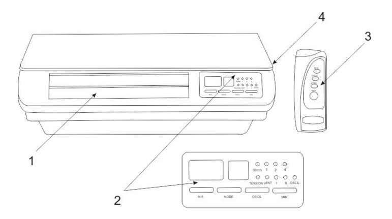
• The following time intervals can be selected: 0,5/1,5/2/2,5/3/3,5/4/4,5/5/5,5/6/6,5/7/7,5 hours. After selection the corresponding LED will illuminate. When the time interval is selected, the countdown will start. The appliance will stop operation and go to the sleep mode, when the selected time is expired.
