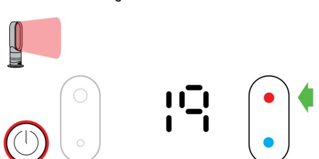
Press the red thermostat control button until the digital display shows the desired target temperature. The power button light will change from blue to red.
