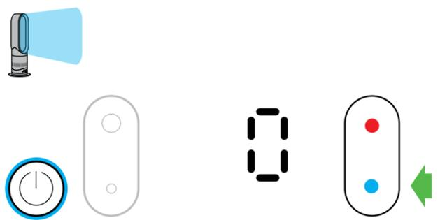
Press the blue thermostat control button to change the target temperature to 0°C. The power button light will change from red to blue. To adjust the airflow speed use the airflow speed control.
