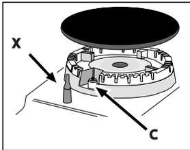
If the appliance is fitted with an electronic lighting device\* (C), press the ignition button, marked with the symbol
