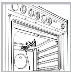
2. Unscrew the grill burner nozzle using a special nozzle socket spanner (see figure) or preferably with a 7 mm socket spanner, and replace it with a new nozzle that is suited to the new type of gas (see *Burner and nozzle specifications table*).
