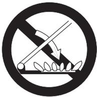
**WARNING!** The glass lid can break in if it is heated up. Turn off all the burners and the electric plates before closing the lid. \*Applies to the models with glass cover only.
