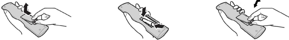
**Note:** If the RC doesn't react to pressing the buttons or the working range was decreased insert the new batteries.
