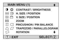
2 To select a control you want to adjust, press the arrow buttons on the front control panel of your monitor and scroll through the choices. When the control you want is highlighted, press button [2].
