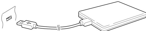
Connect a removable hard drive to one of the receiver's USB ports. For details on how to manage removable storage devices, see Managing Storage Devices on page 35.
