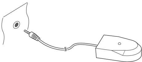
Connect the remote control extender to the **IR Rec.** socket on the receiver. Make sure that the extender does not face directly into light sources, such as lamps or displays. Directing light at the extender may interfere with remote control signal transmission.
