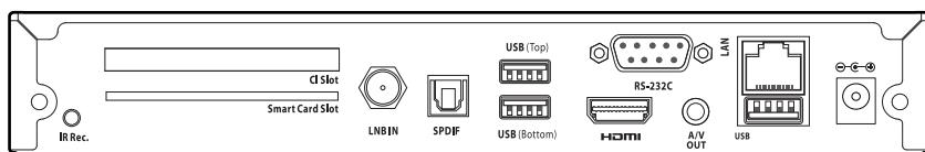
The RS-232C port may be used only by an engineer for installation or service.
