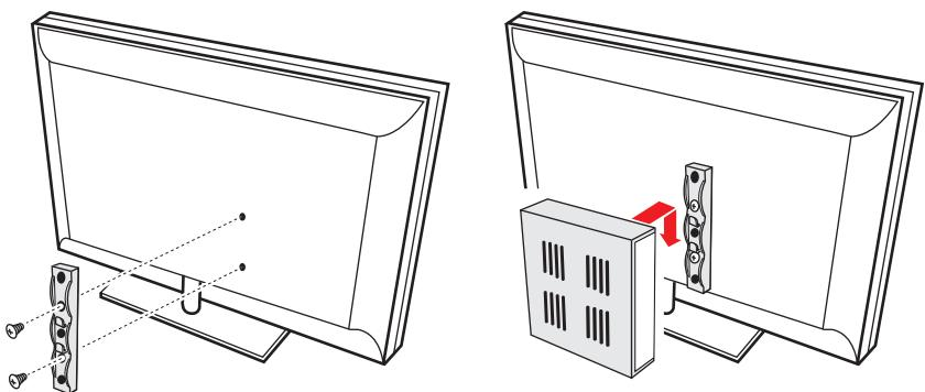
If necessary, mount the receiver on the TV to save space. Install the TV mount bracket on the back of the TV, and then attach the receiver to the bracket, as illustrated by the drawings above.
