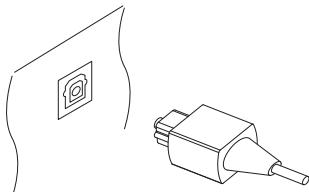
Use an AV receiver for better audio quality. Connect the receiver's SPDIF connector to the AV receiver's digital audio input connector using an optical audio cable.
