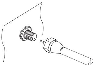
Connect the cable from the satellite dish to LNB IN.
