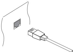
Connect the receiver's LAN port to the router using a network cable. For details on how to configure the network settings, see Network Settings on page 50.
