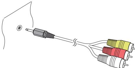
Insert a jack-to-RCA cable's jack into the A/V OUT socket on the receiver, then insert the RCA plugs on the other end into the TV's composite video and audio input sockets. Make sure to match the connectors' colours properly.
