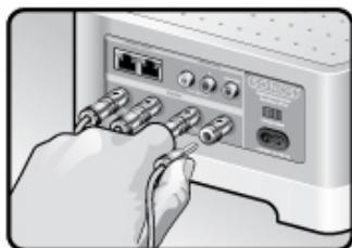
If your speakers have banana connectors, you can insert the plugs directly into the banana jacks on the back of the CONNECT (available in North America only).
