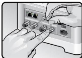
If you are using speaker wire, use your finger to firmly push the spring-loaded speaker post to reveal the connection hole.
