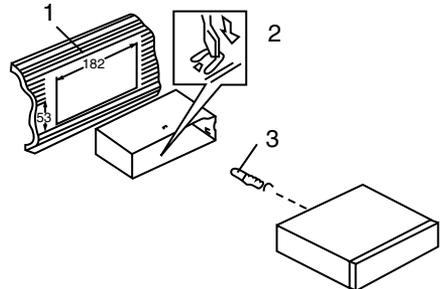
1. Install the sleeve into the dashboard; ensure it is installed with the correct side and there are no obstacles (wires, dashboard elements, etc) for the unit installation.
