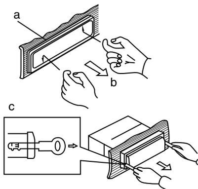
1. Switch off the unit and detach the front panel.
