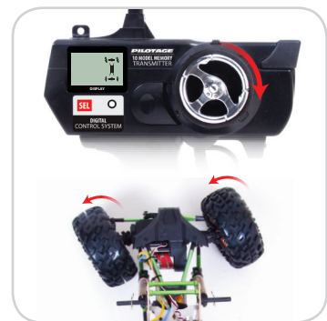
Reversed steering response (incorrect directional response)
