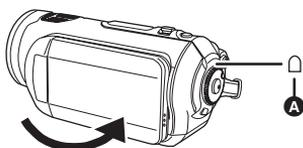
The status indicator **A** goes off and the power turns off. (If [QUICK START] is set to [ON], the unit goes into quick start standby mode and the status indicator lights green.)
