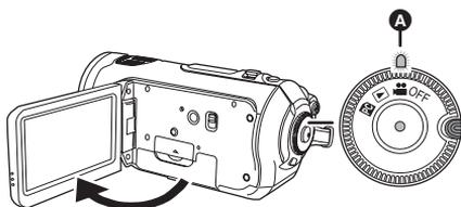
The status indicator **A** lights red and the unit is put into recording pause approx. 1.7 seconds after it is turned on.
