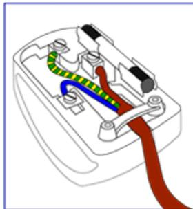
1. The GREEN AND YELLOW wire must be connected to the terminal in the plug which is marked with the letter "G" or by the Ground symbol  $\perp$  or coloured GREEN or GREEN AND YELLOW.
