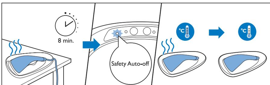
**EN** Press the steam trigger to let the steamer reheat.
