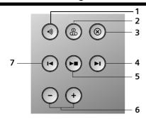
You can use the keys on the base unit to operate the built-in answering machine and register handsets to the base.
