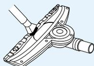
1. Remove dusts accumulated where the floor surface of the suction hole for device protection is dirty.
