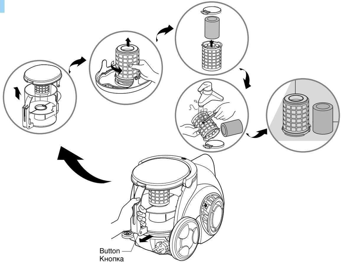
The reusable motor filter is situated under the dust chamber cap and you can use it permanently.
