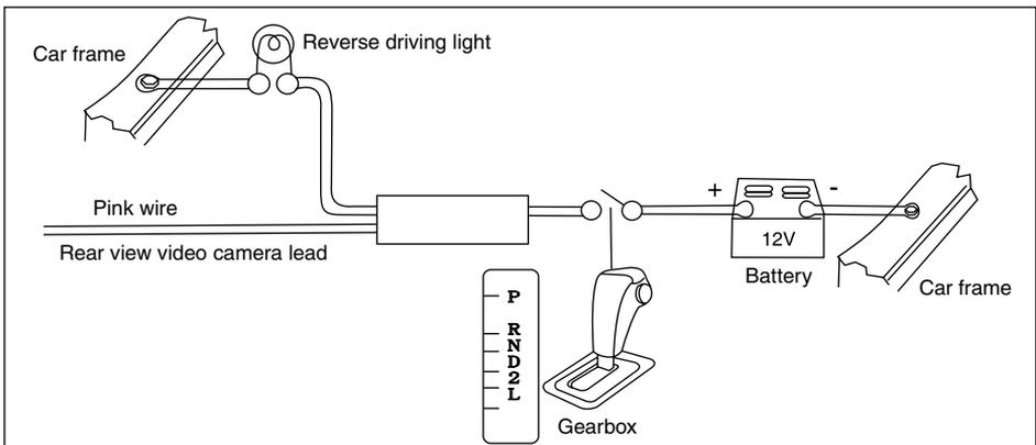
If the rear view video camera is connected, the unit automatically switches to camera mode during reverse driving. The unit returns to the original work mode after the reverse driving is done.
