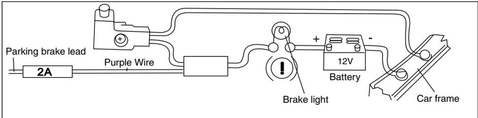
If Parking cable is connected to hand brake switch, the video display of the TFT monitor will be controlled by driving status. When the car is moving ahead, if the video disc is played, the screen shows warning and blank screen. The warning screen will prevent the driver from watching images.
